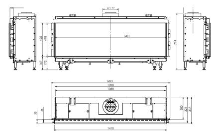
The balanced flue components themselves must be taken into account and connecting to the appliance itself (we call this the 'heat engine') via the spigot on top. These components will either exit from an outside wall, at least one metre above the heat engine, or will go vertically through the building and exit the roof:
