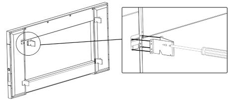
Before fitting the fascia, the hooks must be attached using the screws supplied. The ESCEA EW5000 fascia is attached to the firebox by four 'hooks' on the corners of the fascia.
