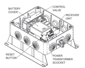
To connect the UF95ORCS to 240v mains electricity instead of using batteries for ignition, you should do so using the transformer supplied.
