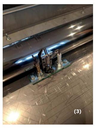
Do not put any strain on the thermocouple or ignition lead.
