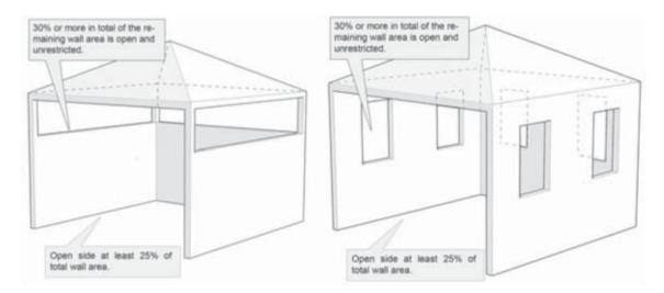
6.3 Rectangular areas have been used in the above diagrams for illustrative purposes; the same principles apply to any other shaped area. In the case of balconies, at least 20% of the total wall area should be and remain open and unrestricted in use.
