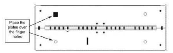
TIP: Use the finger holes to easily remove the burner assembly from the masonry cutout or burner tray.
