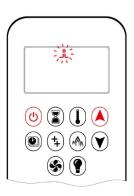
(3) Now release the On/Off button. The ignition procedure has been started.
